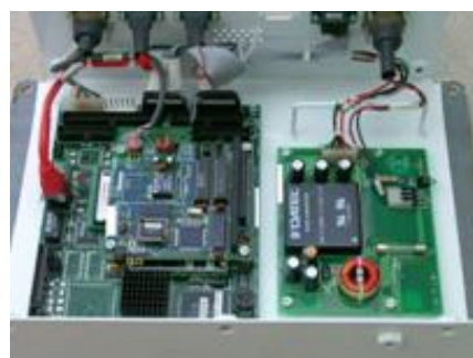
Figure 4: GPS card and industrial PC cards.
